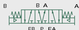
double air pilot 3 Position 4-Way (5/3), open to 4 (A) and 2 (B) in center
