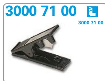
This tool will cut all resilient plastic tube (nylon, FEP, polyurethane, braided PVC) from 4mm to 14mm diameter inclusive. It is designed to give a clean cut at right angles to the tube axis. A spring maintains the cutter in the closed position.
