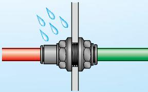
All plastic nuts are fitted with an integral O-ring to optimise sealing to a bulkhead wall.
